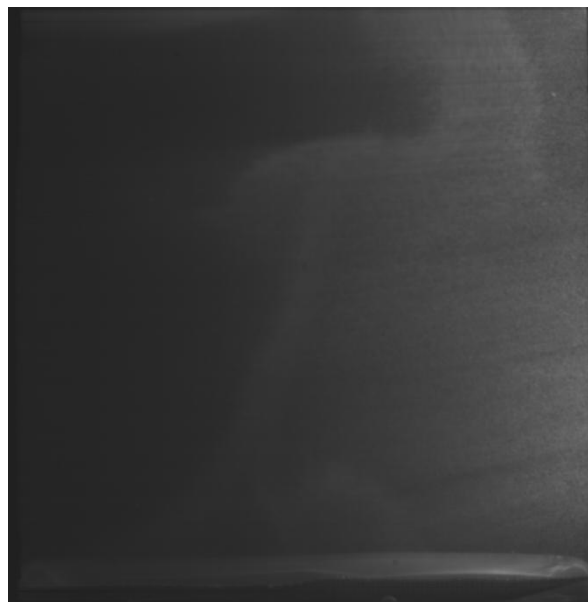
Figure 5.7: 'Fluidised' G100FF - loose sample. Note lighter areas where surges of oil are flowing, therefore having a lower density of particles.
