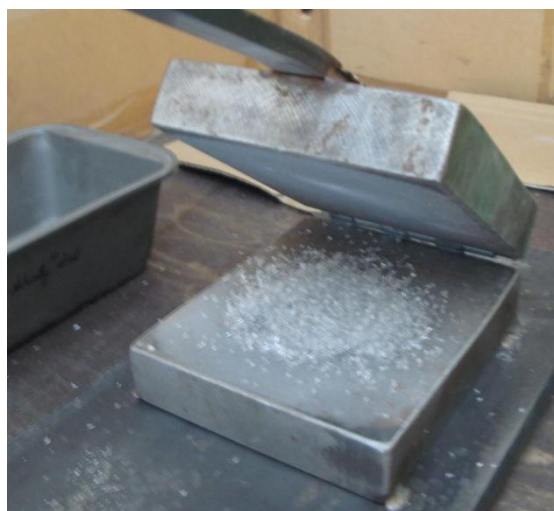
Figure 4.16: Steel slabs used for crushing the glass tubing to make fine particles.
