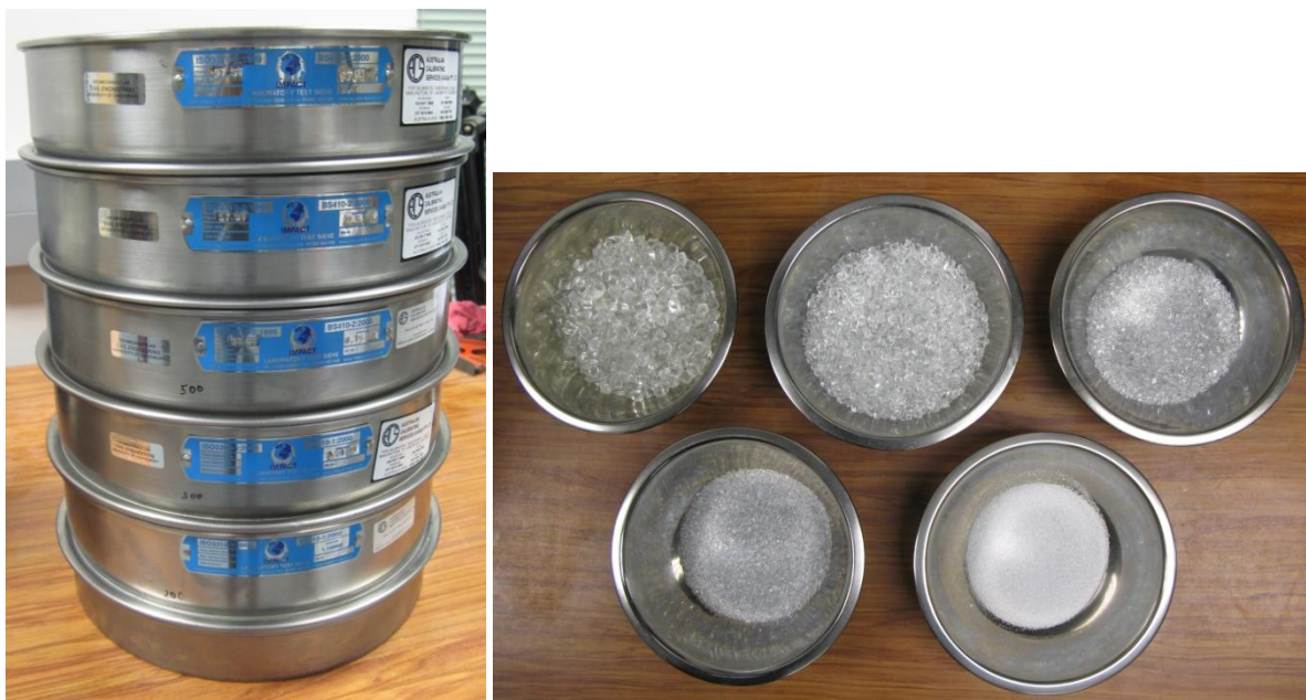
Figure 4.21: Clean glass particles are sieved and separated into like particles sizes, ready for the creation of a different PSD.
