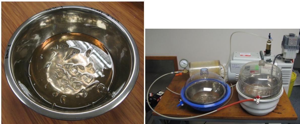
Figure 4.22: a) oil is added to the glass PSD and then; b) the glass particle-oil mixtures are placed into vacuum desiccators.
