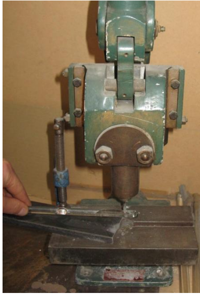
Figure 4.17: Bench machine used for producing larger particles by cutting the glass rods.
