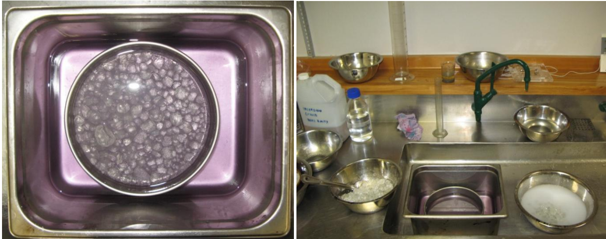
Figure 4.20: Glass particles being washed in methyated spirits bath. Particles are then poured into water before rinsing through a sieve.
