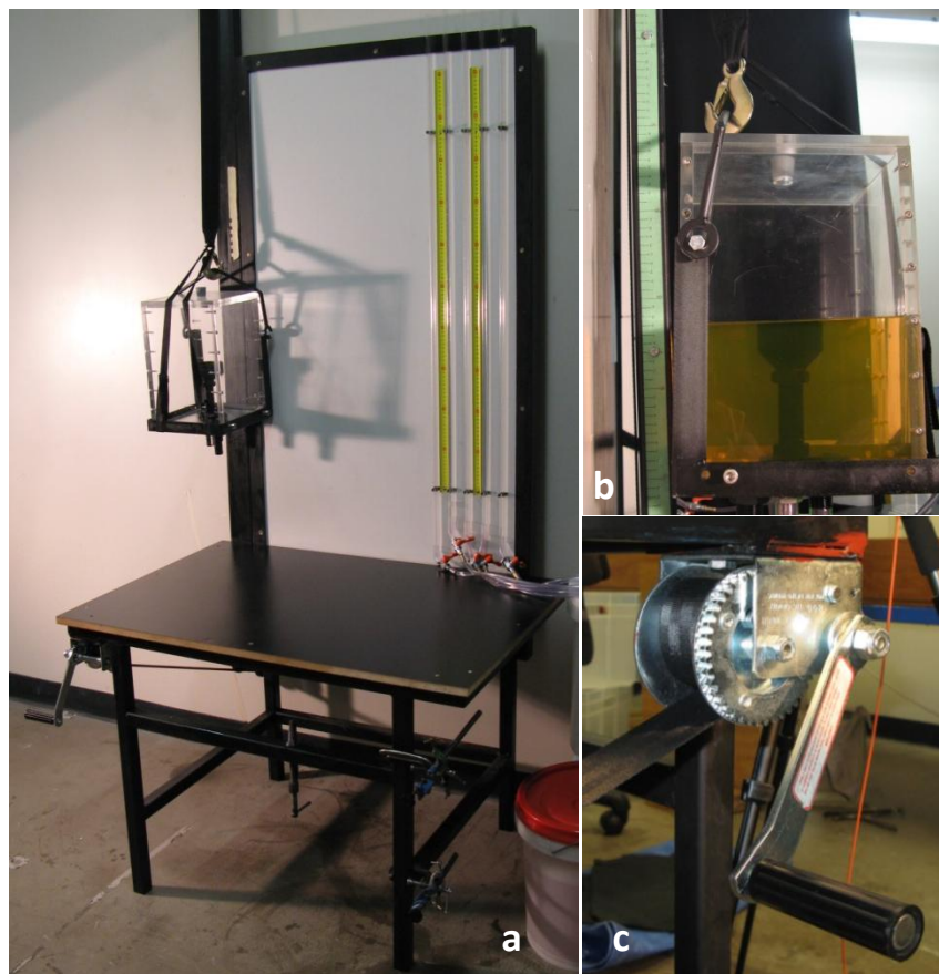
Figure 4.33: Oil control system: a) Bench with attached hand winch, header tank and piezometer tubes; b) header tank with height scale; c) hand winch to control head.
