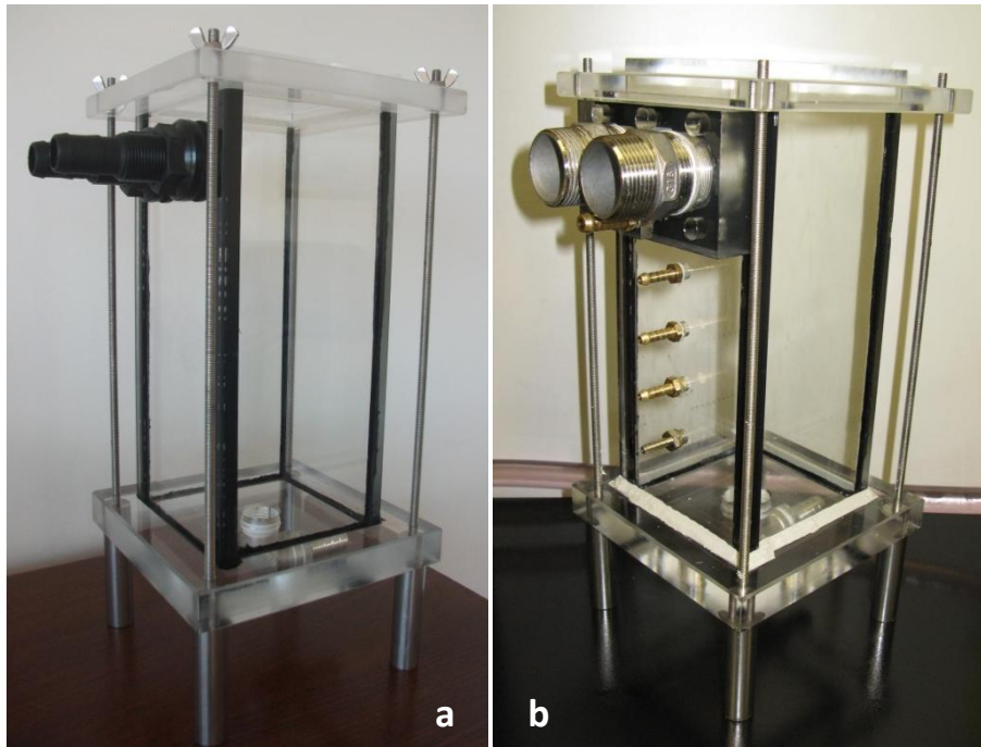
Figure 4.27: a) Original apparatus before modification – note 2x 15 mm \varnothing outlet ports and; b) Apparatus after modifications - note increase in port to 40 mm \varnothing , a total of 5 piezometer ports, additional silicon sealant around base.
