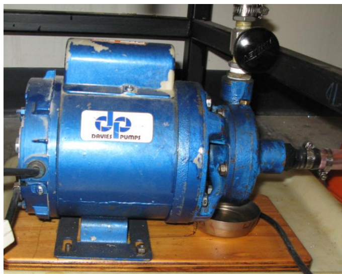
Figure 4.30: Davies and Onga Pump used to pump oil into header tank.
